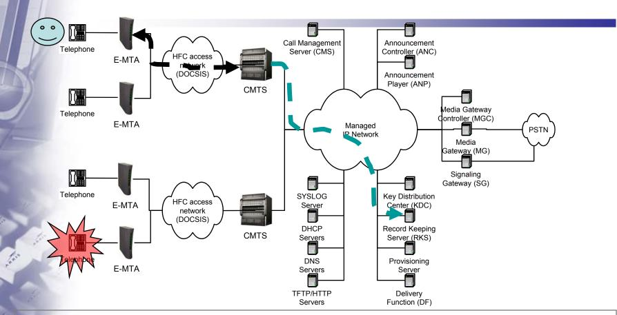
MTA<sub>o</sub> uses a DOCSIS Dynamic Services transaction to create an admitted upstream flow and an admitted and activated downstream service flow using Gate-ID<sub>o</sub>. CMTS<sub>o</sub> sends an upstream QoS-Reserve and downstream QoS-Reserve and QoS-Commit event messages to the RKS.
