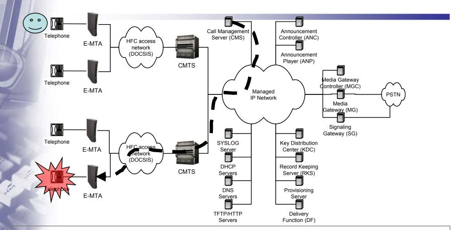
CMS creates an inactive connection on  $MTA_T$  and passes the Gate-ID<sub>T</sub> that it received in the previous step. CMS instructs  $MTA_T$  to ring the phone and asks for notification when the call is answered.
