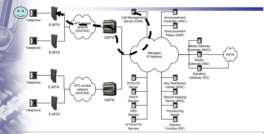
CMS creates an inactive connection on MTA<sub>o</sub>. CMS tells MTA<sub>o</sub> to look for onhook, play dialtone and collect digits according to digit map.
