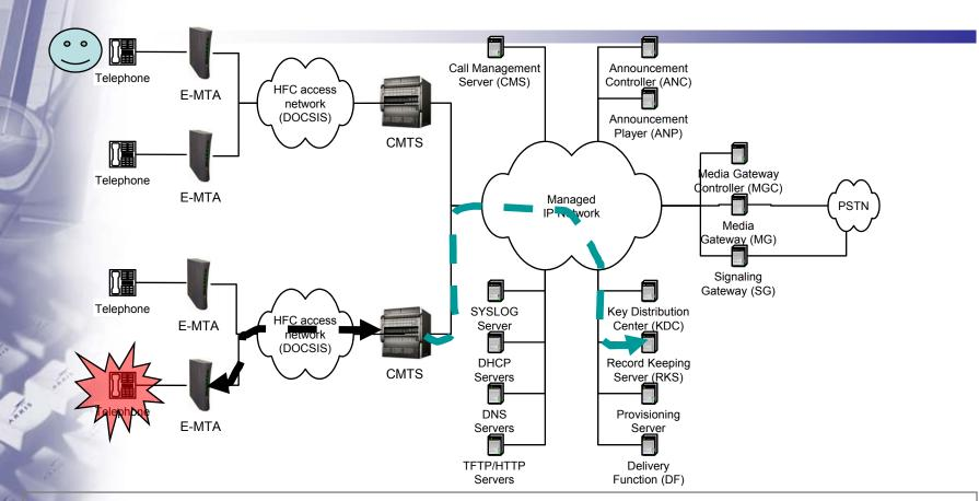
Meanwhile,  $MTA_T$  uses a DOCSIS Dynamic Services transaction to create admitted upstream and downstream service flows using Gate-ID<sub>T</sub>. CMTS<sub>T</sub> sends upstream and downstream QoS-Reserve event messages to the RKS.
