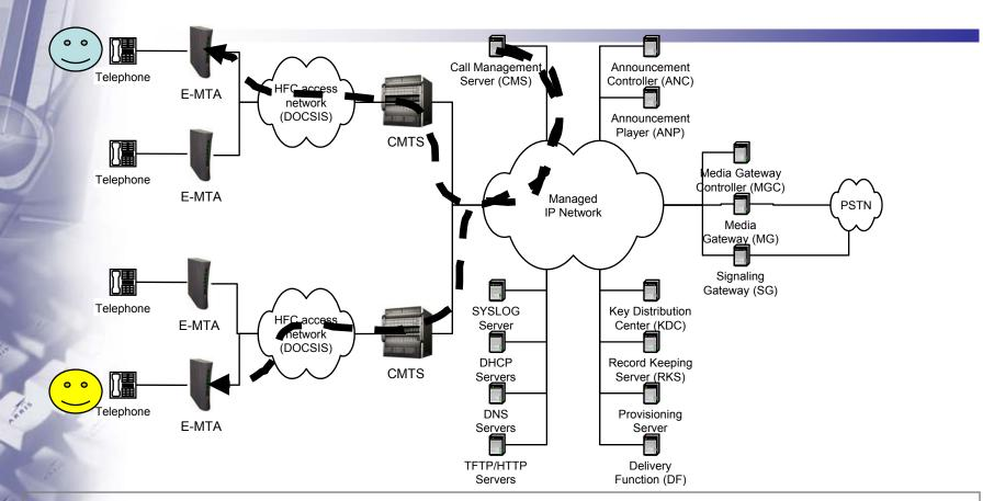
Nearly simultaneously, the CMS instructs both  $MTA_o$  and  $MTA_T$  to change their connections to send-receive mode. CMS tells  $MTA_T$  to look for onhook.
